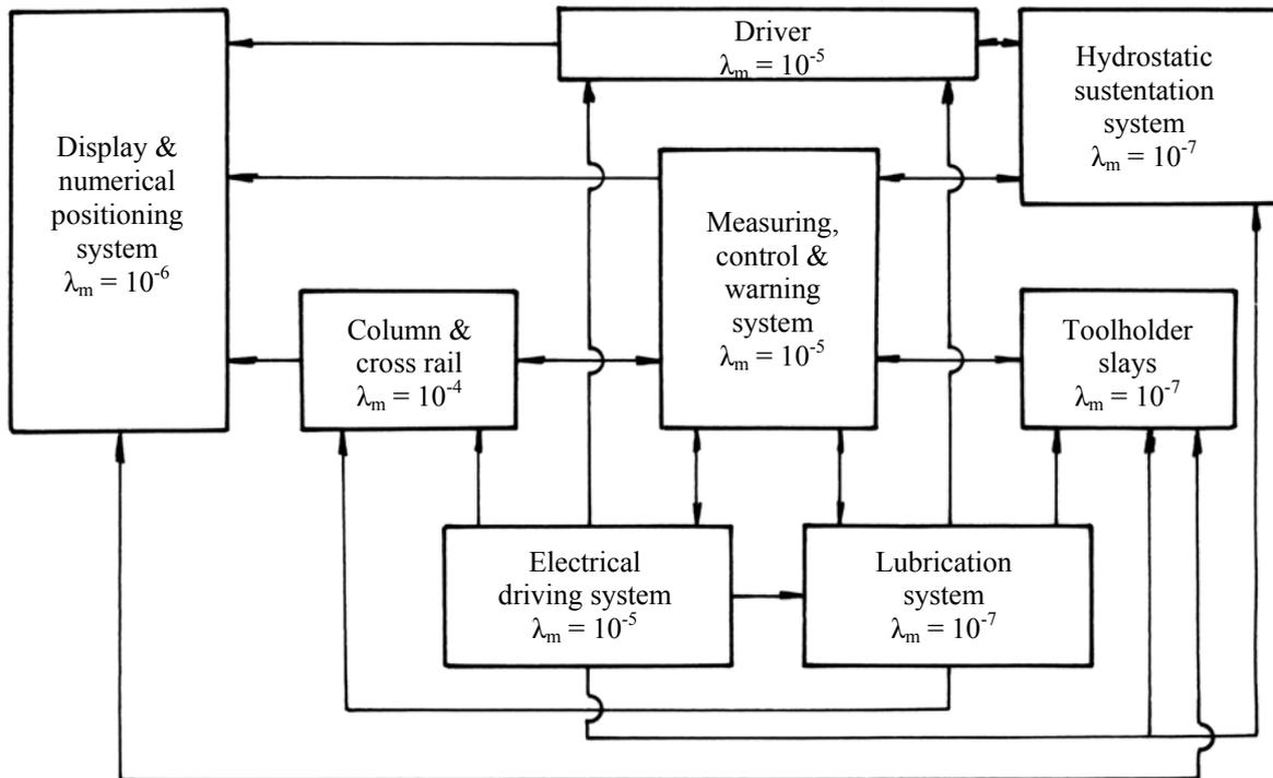
Fig. 3. Interconnections in assessing a vertical lathe reliability
